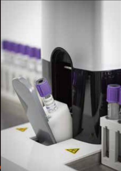
STAT position Easy switch from autoloader loader
