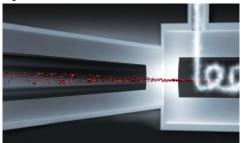
The DynaHelix Flow technology perfectly aligns WBC, RBC and PLT cells for high impedance counting precision using advanced hydrodynamic-focused sheath flow before passing through the aperture. In addition, the DynaHelix Flow totally prevent risk of coincidence or count of blood cell re-entry into the aperture using unique DynaHelix Flow stream. This newly-developed advanced DynaHelix Flow technology greatly improve counting precision and accuracy.
