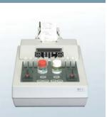
The BFT II Analyzer is a semi-automated device intended for in vitro diagnostic use to determine PT, APTT, Fibrinogen, Thrombin time, Batroxobin time, single factors, Lupus anticoagulant, Protein C and Factor V Leiden.
